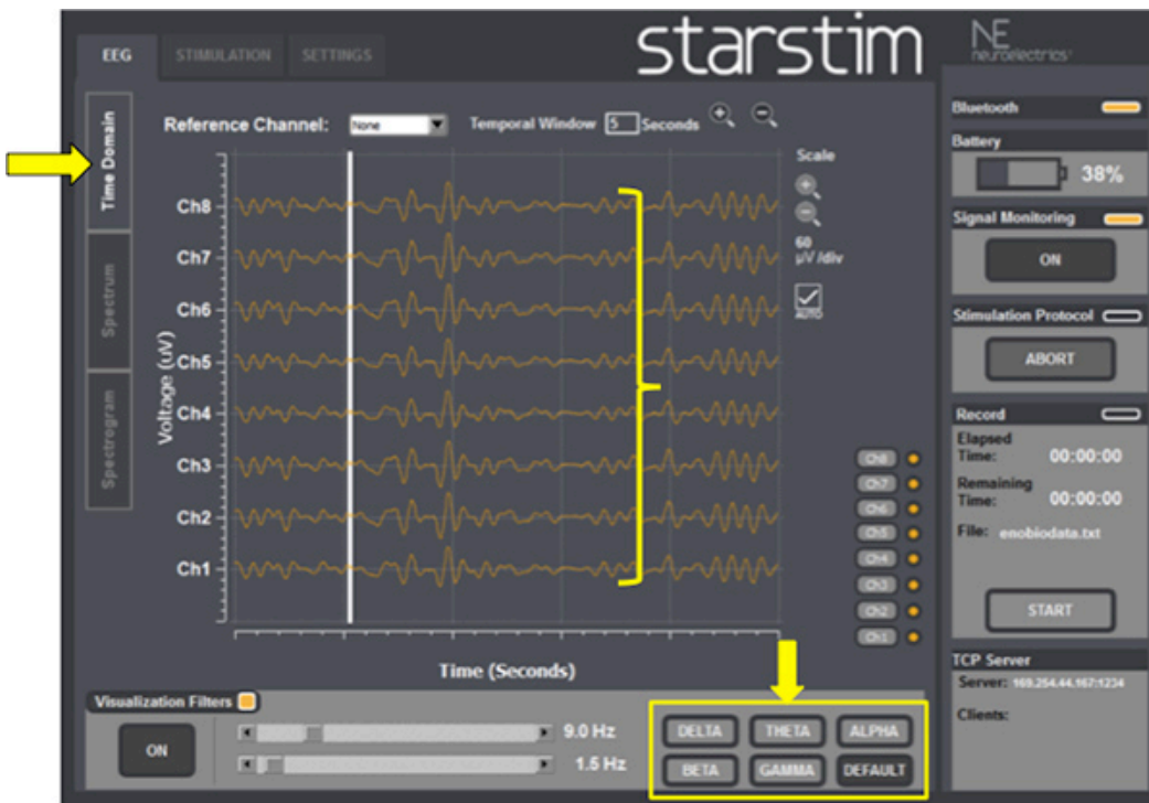
Figure 6. EEG Time domain: check the baseline ongoing EEG activity and select EEG band frequencies if needed (yellow arrow at the right bottom).
